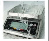
\*IP68 waterproofness means that it is also fully dustproof and that its waterproof performance can be maintained even when the instrument is laced underwater at a depth of 1 meter for 24 continuous hours.
